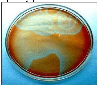
Belousov-Zhabotinskii type reaction giving rise to three-dimensional channel’s waves
